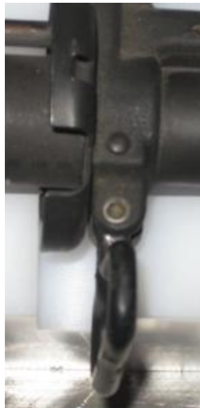
Figure 55: Riveted Sling swivel, grind or drill to remove.
