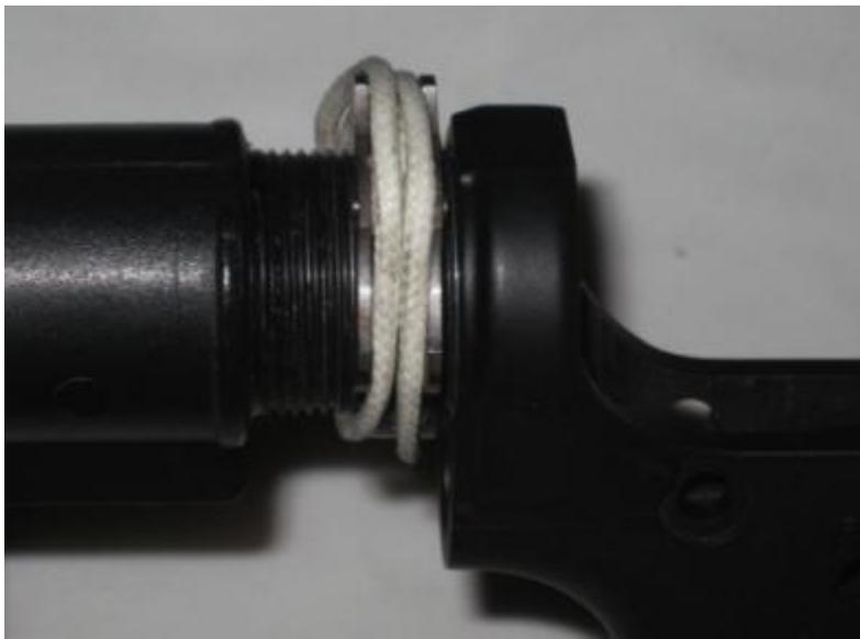
Figure 40: Use of Strap Wrench Accessory to tighten CAR stock nut
