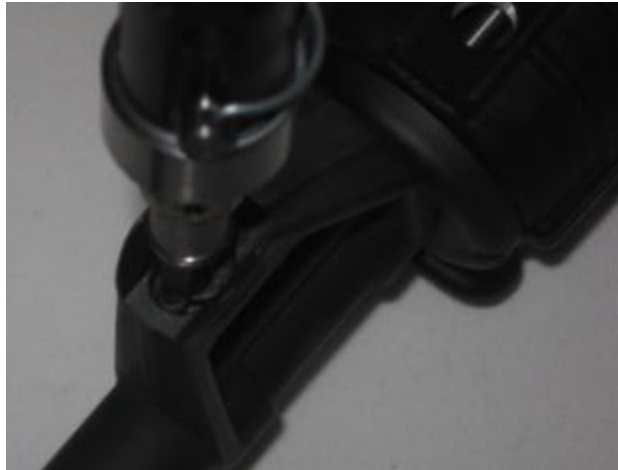
Figure 43: Front Sight Bit used in Screwdriver Mode.
