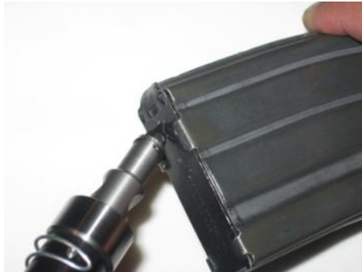
Figure 58: Lift Magazine Floor Plate
