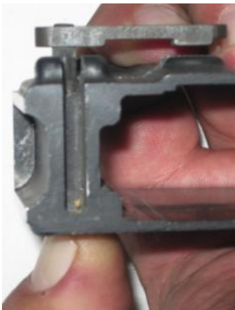
Figure 31: Depress Magazine release Button flush with receiver.
