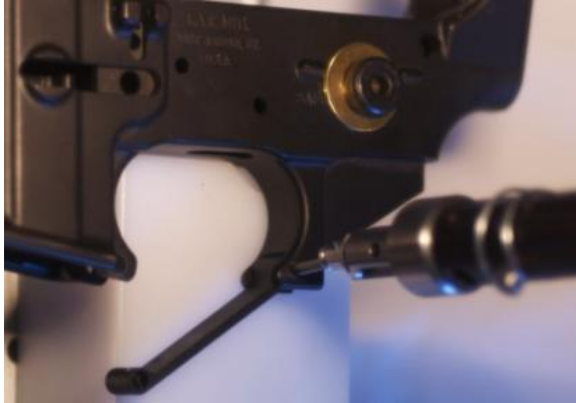
Figure 15: Installing Trigger Guard
