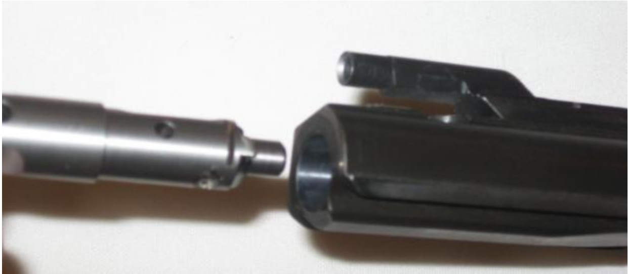
Figure 62: Bolt Carrier carbon may be scraped using the scraper body.
