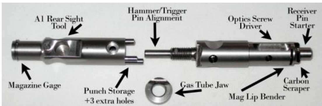
Figure 2: Inner Sub Assembly Function and Components
