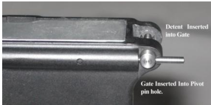
Figure 17: Use of the Gate to install Front Pivot Pin
