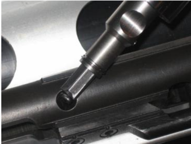
Figure 64: Remove Bolt Carrier Cotter Key with Front sight Tool
