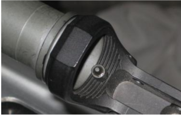
Figure 33: Buffer Tube retaining plunger installed onto spring
