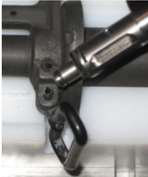
Figure 54: Sling Swivel installation/removal
