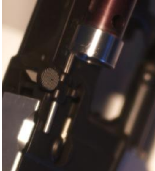
Figure 27: Roll Pin in Torque Body, inserted into Bolt Release
