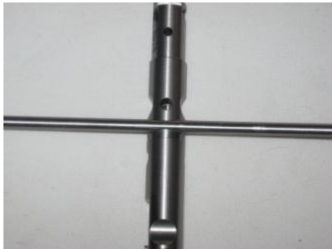
Figure 47: The gas tube is clamped between scraper and driver bodies using the gas tube wrench washer.
