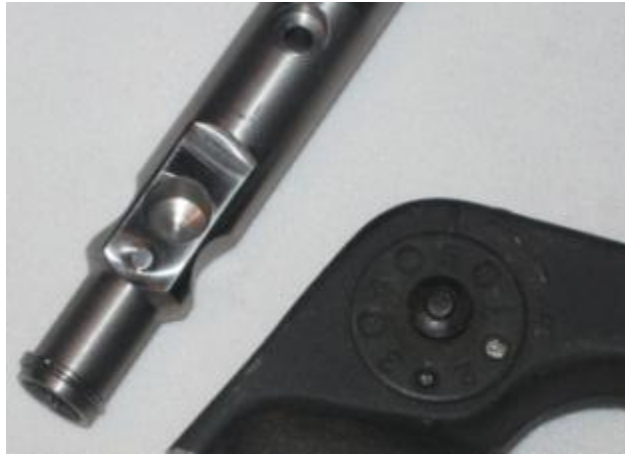
Figure 44: A1 Rear Sight Adjustment tool
