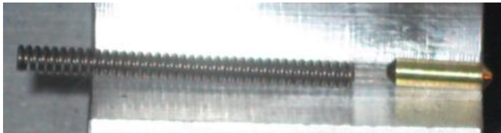
Figure 18: Spring and Detent for front pivot Pin:
