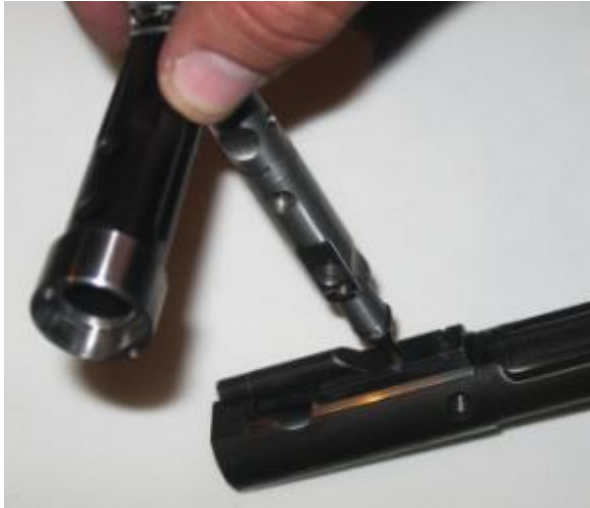
Figure 56: Gas Key Screw installation/removal
