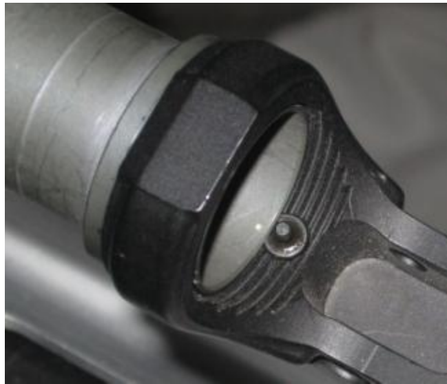
Figure 34: Buffer tube screwed in to receiver, capturing buffer tube retaining plunger.
