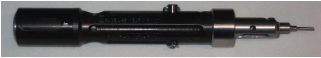
Figure 7: Punch Mode with 1/16" punch
