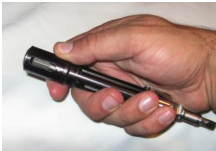
Figure 11: Alternative method to remove bits from the bit magazine
