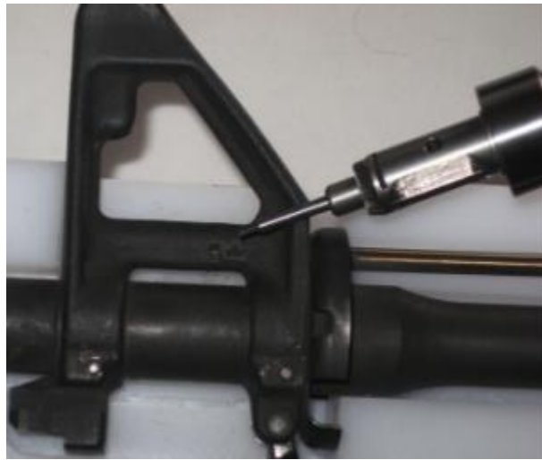
Figure 48: Installation/Removal of the gas tube retaining roll pin.
