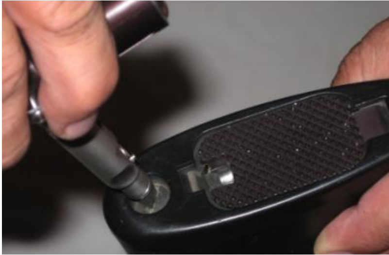
Figure 39: Screwdriver Mode to remove butt plate on fixed stock
