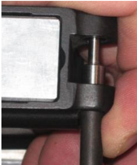
Figure 21: Pivot Pin is driven in to push the gate out.
