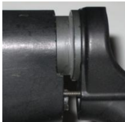
Figure 38: Slide Stock on Buffer Tube to capture spring
