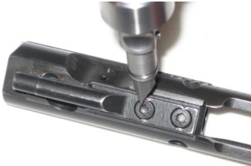
Figure 57: Staking Gas Key Screws
