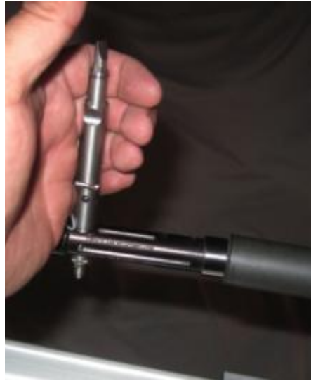
Figure 35: Torque handle being used to tighten buffer tube.
