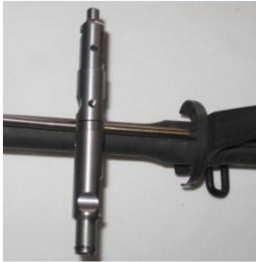
Figure 46: Gas Tube Removal: Clamped between scraper and driver bodies.
