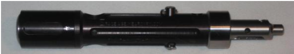
Figure 8: Punch Mode without Punch installed
