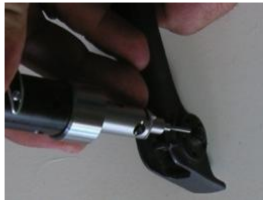
Figure 42: Rear Sight Roll Pin installation
