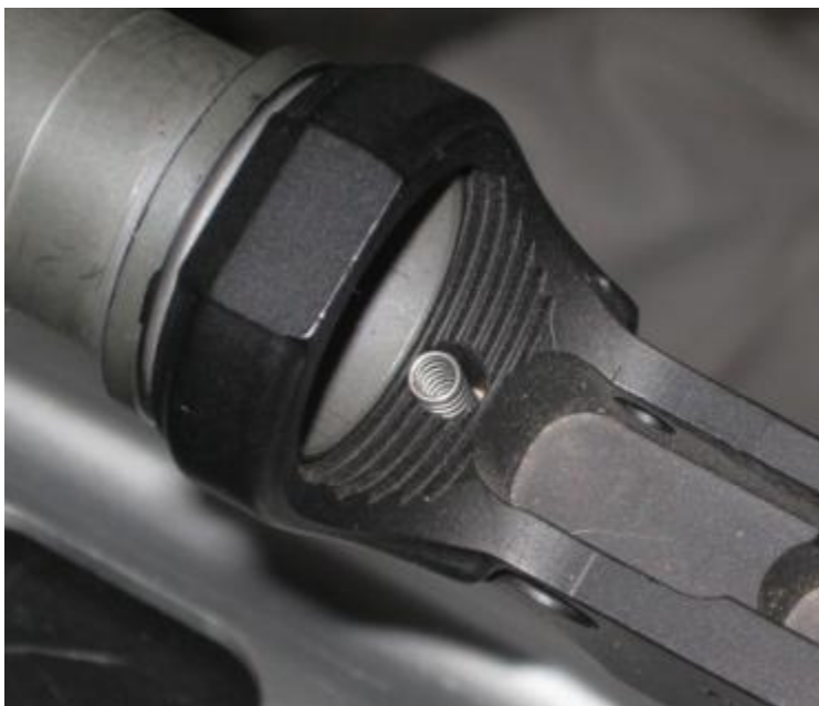
Figure 32: Buffer Tube Plunger Spring installed into lower Receiver.
