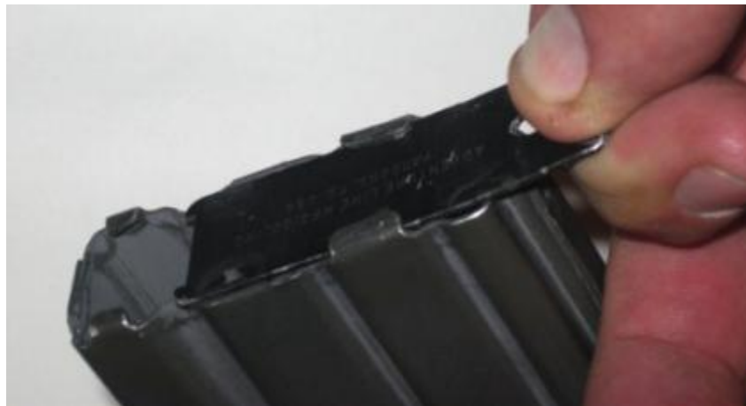
Figure 59: Finish Removal of Magazine Floor Plate
