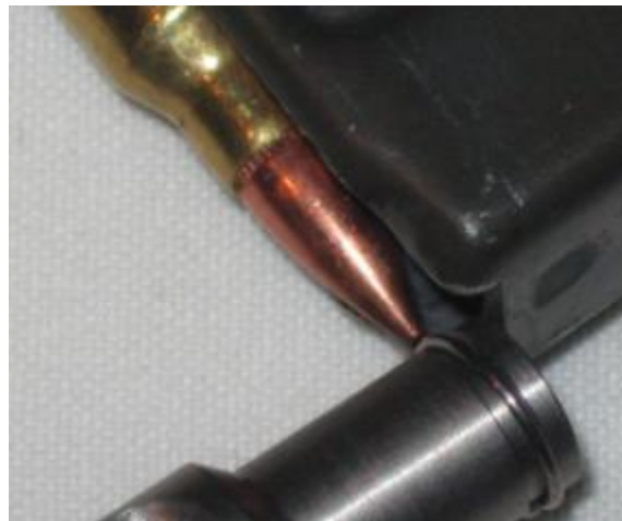
Figure 61: Magazine Lip Gauge use: Bullet tip should align on retention spring.
