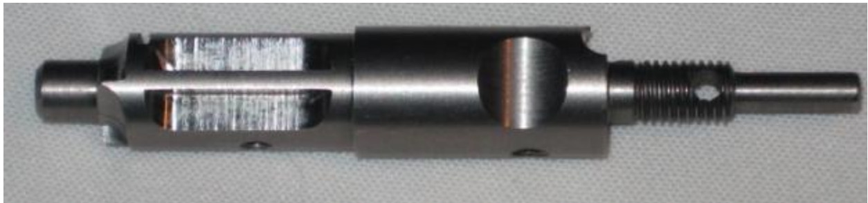
Figure 24: Scraper body, with Hammer/Trigger Pin Driver & alignment punch
