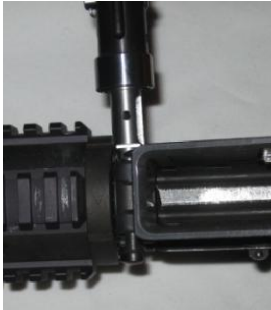
Figure 23: Punch body is used to push out sticky receiver pins
