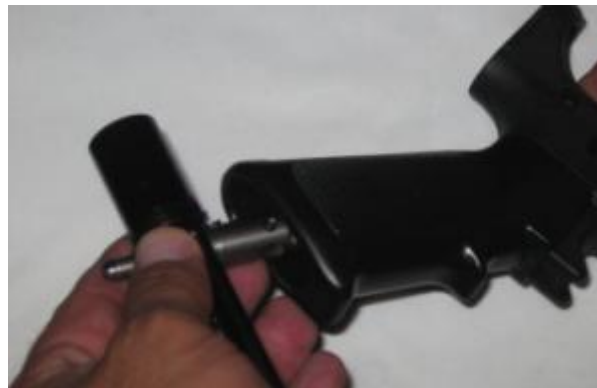
Figure 28: Tee Handle Mode to tighten Pistol Grip
