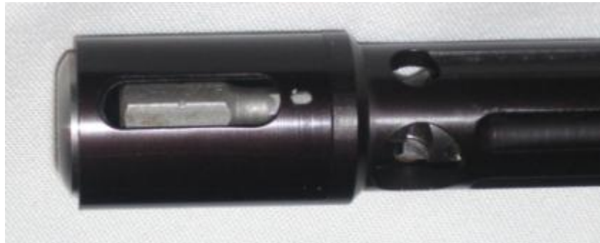
Figure 10: Bit magazine with hex bit properly inserted
